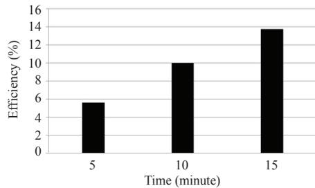
**Figure 12:** The efficiency of pressing palm at a speed of 155 rpm after dried with hot air.
