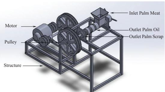
**Figure 2:** The plan of palm oil pressing machine.
