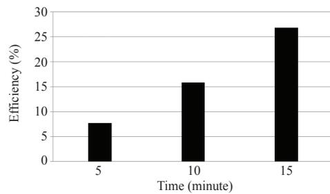
**Figure 8:** The efficiency of pressing palm at a speed of 133 rpm before dried with hot air.
