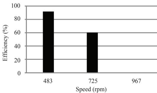
**Figure 6:** The chart of the efficiency of palm seeds separation at various speeds.
