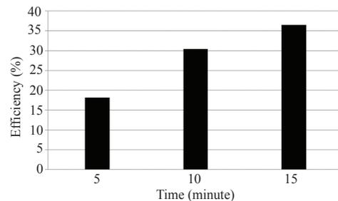
**Figure 9:** The efficiency of pressing palm at a speed of 155 rpm before dried with hot air.
