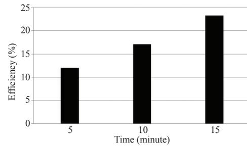
**Figure 7:** The efficiency of pressing palm at a speed of 110 rpm before dried with hot air.
