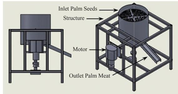
**Figure 1:** Palm seed separating machine plan.
