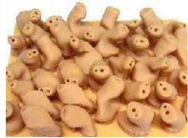
Figure 3: Individually customized hearing aid shells mass-produced by an EOS laser sintering system. Special CAD software has been developed by Materialize to make the process of converting the customers' ear canal laser scan data into the product easy and seamless.
