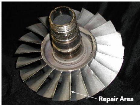
Figure 9: Example of repaired blisk for T700 jet engine, [4].
