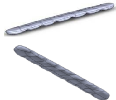
Figure 6: CAD model of the LENS fixation plate prototype
