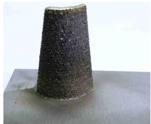
Figure 12: Final shape of the individual testing blisk blade
