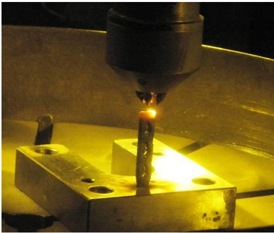
Figure 7: Manufacturing of the fixation plate prototype on Optomec LENS 850R machine
