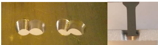
Figure 8: Machined screw holes and intentionally developed cutting tool
