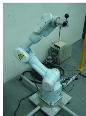
Figure 9: PA10-7C manipulator arm with a spherical target
