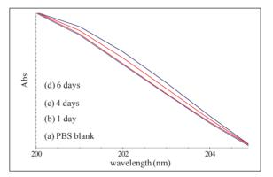
**Figure 7**: UV-Vis spectra of P-P-I-T fiber mats as a function of degradation time: 1, 4, and 6 days.
