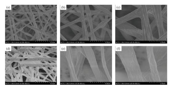
**Figure 2**: SEM images of electrospun fibers (a)–(c) P-P-T and (d)–(f) P-P-I-T at 5,000×, 10,000×, and 20,000× magnifications.
