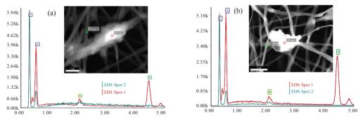
**Figure 3**: EDX spectra illustrating atomic compositions of bead defects with different sizes present in (a) P-P-T and (b) P-P-I-T fibers.
