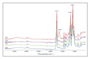
**Figure 6**: ATR-FTIR spectra of electrospun P-P-I-T (10 kV) fiber soaked in PBS solution at: (a) 0, (b) 1, (c) 4, and (d) 6 days.
