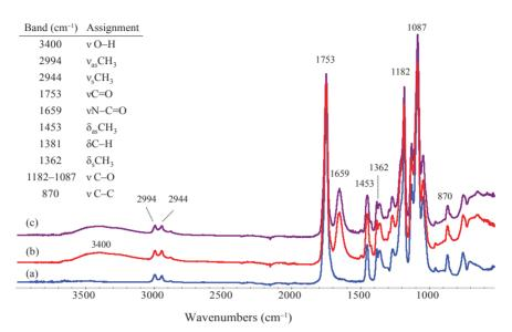
Figure 1: ATR-FTIR spectra of fiber mats: (a) Neat PLA, (b) P-P-T, and (c) P-P-I-T.
