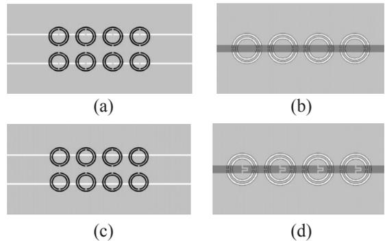
Figure 5: CPW structure: (a) loaded pairs of SRRs with shunt metal strips [53], (b) loaded array of CSRRs [54], (c) loaded pairs of SRRs [55], [56], and (d) loaded an array of CSRRs [55].
