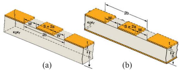
**Figure 1:** Coplanar waveguide structure: (a) not ground-backed [16] and (b) with ground-backed [16].
