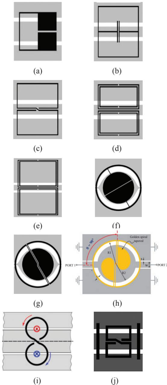
**Figure 7:** CPW structure: (a) loaded with symmetric folded SIR [58], [59], (b) ELC SRR [8], [59], [60], (c) square S-shaped SRR [60], (d) pair of rectangular SRRs [60], (E) pair of square SRRs [60], (f) ELC tapered SRR [8], [60], (g) S-shaped tapered SRR [60], (h) S-shaped golden spiral-tapered SRR [23], (i) S-shaped SRR [20], and (j) rectangular S-shaped SRR [20].
