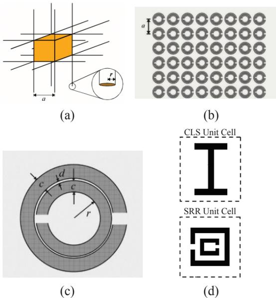
**Figure 2:** Split ring resonator structures: (a) periodic structure of copper wire [35], (b) SRR in square array [36], (c) top view of SRR [36], [37], and (d) combination between CLSs and square SRRs [38].
