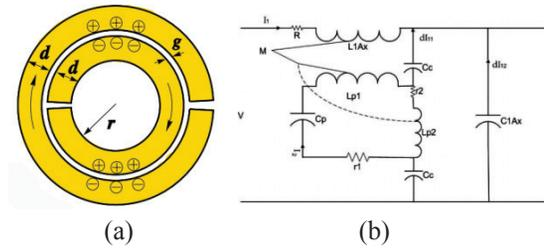
**Figure 3:** Single SRR: (a) double circular SRR and (b) equivalent circuit of SRR [39].
