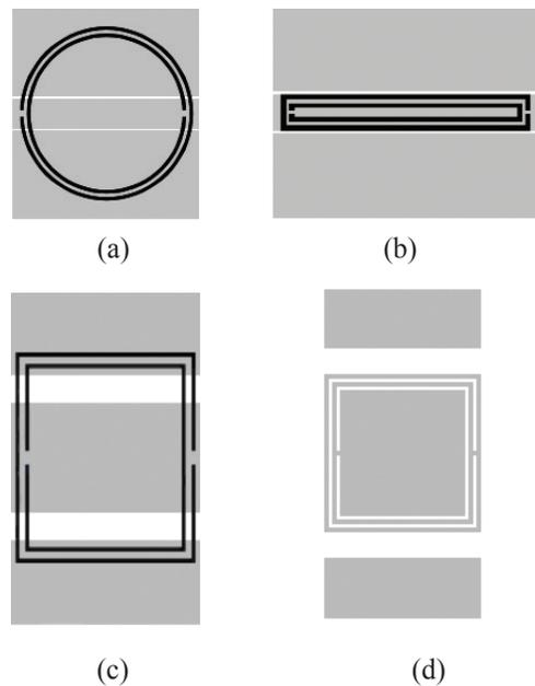
Figure 6: CPW structure: (a) symmetric circular-shaped SRR [22], (b) symmetric rectangular-shaped SRR [22], (c) symmetric square-shaped SRR [22], [57], and (d) symmetric square-shaped CSRR [57].
