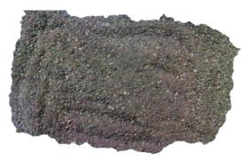
**Figure 4**: Milled plantain peel retained on U.S. standard sieve size number 50 (0.30 mm opening).
