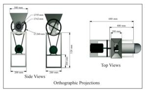
**Figure 2**: Orthographic projections of the varying dieplate fish feed pelletizer.
