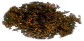
Figure 7: Formed pellets from the 5 mm die plate.
