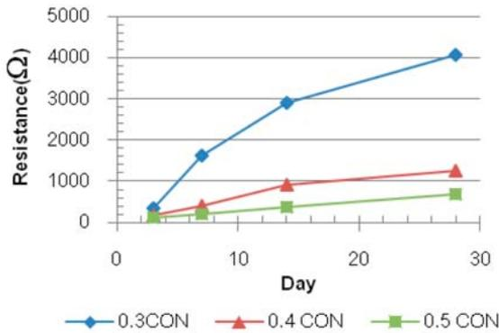
**Figure 4:** Resistivity of the sensors made of plain cement paste having the w/b ratio of 0.3, 0.4, and 0.5.
