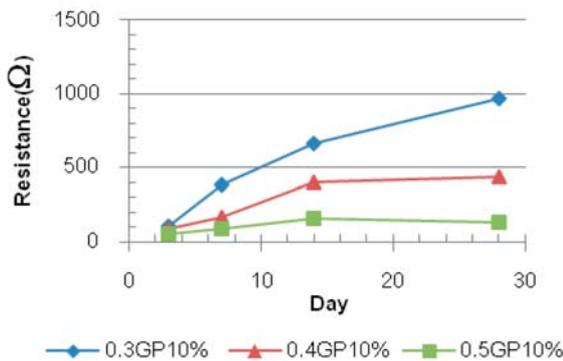
**Figure 6:** Resistivity of the sensors made of 10% graphite powder cement paste having the w/b ratio of 0.3, 0.4, and 0.5.
