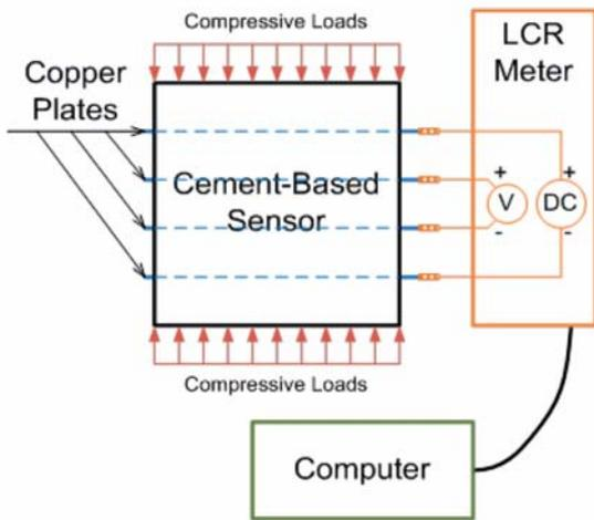
**Figure 2:** Schematic diagram of the connection between the sensor and the LCR meter following the four probe method.
