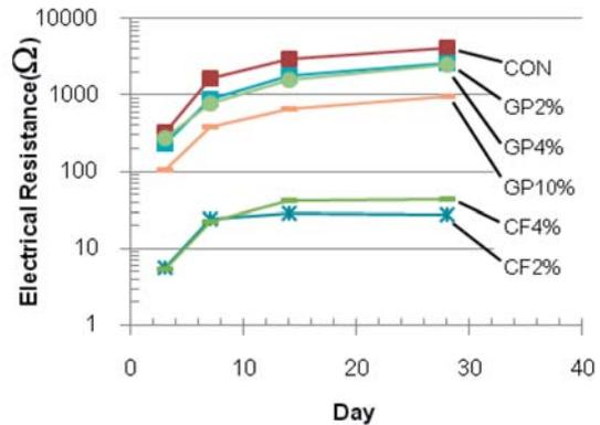
**Figure 3:** Resistivity of the sensors having the w/b ratio of 0.3.
