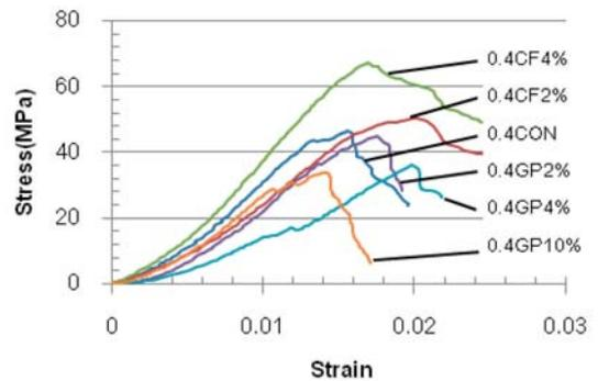
**Figure 8:** Stress-strain relation of the sensors having the w/b ratio of 0.4 under compression test.
