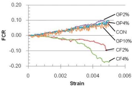
**Figure 10:** Relation of the FCR of the sensors (w/b ratio = 0.3) and compressive strain in the range of 0.005.
