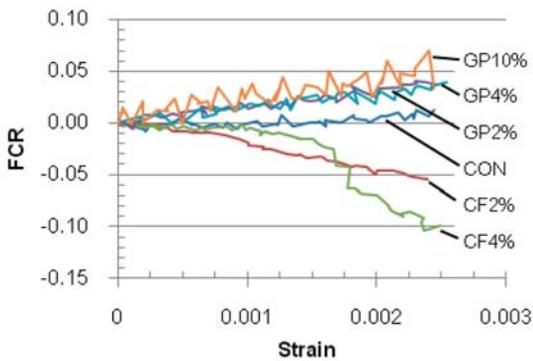
**Figure 9:** Relation of the FCR of the sensors (w/b ratio = 0.3) and compressive strain in the range of 0.0025.
