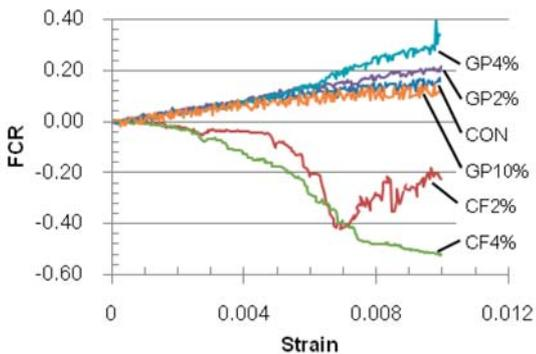
**Figure 11:** Relation of the FCR of the sensors (w/b ratio = 0.3) and compressive strain in the range of 0.01.
