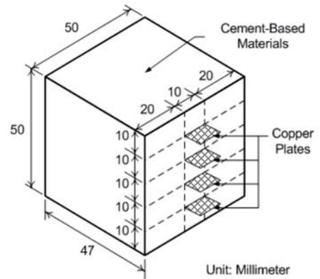
**Figure 1:** Sample of the cement-based sensor.
