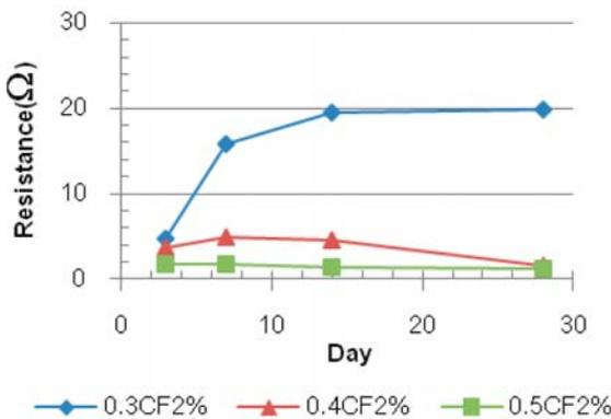
**Figure 5:** Resistivity of the sensors made of 2% carbon fiber cement paste having the w/b ratio of 0.3, 0.4, and 0.5.
