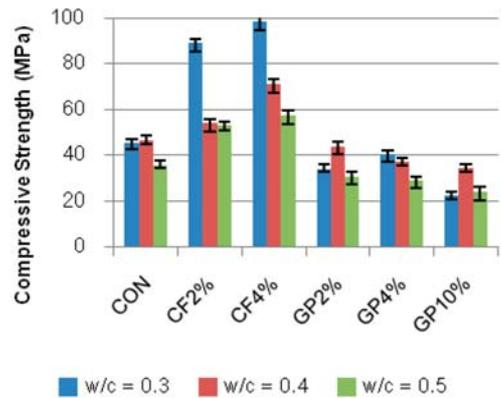
**Figure 7:** Compressive strength of the sensors made of different mixes.
