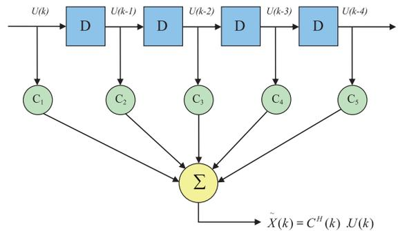
Figure 2: FIR Filter architecture.
