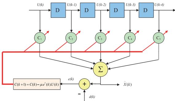
**Figure 3:** Architecture of FIR Filter with LMS adaptation.
