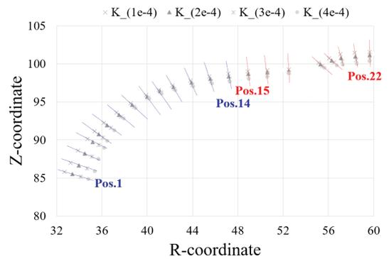
**Figure 20:** Conversion of the wear depth to the cartesian coordinates for each K-values at different positions.
