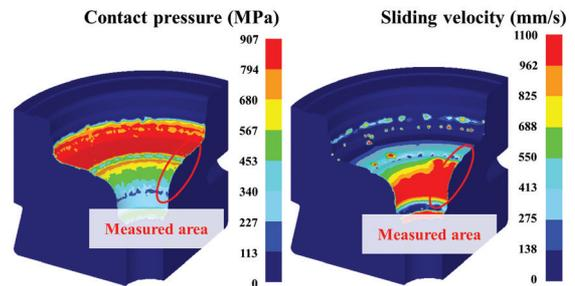
**Figure 16:** Results of the lower die at the finished stage, (a) contact pressure and (b) sliding velocity.
