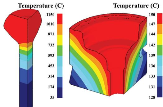
**Figure 11:** Preheated process of workpiece and lower die in FEM.
