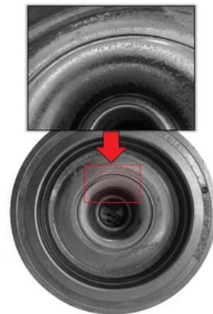
Figure 2: Abrasive wear on the die surface.
