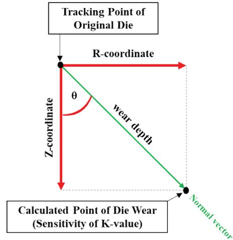
**Figure 5:** Method to convert wear depth for coordinate system.
