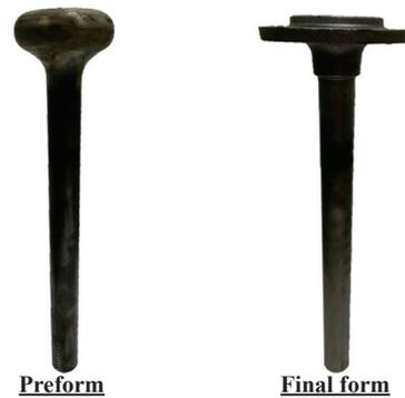
**Figure 8:** Samples of the preform and final form of the product for 3D-scan measurement.
