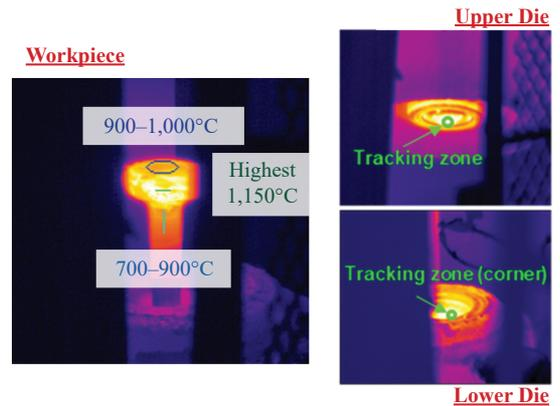
**Figure 7:** thermal images of the workpiece, upper die and lower die.
