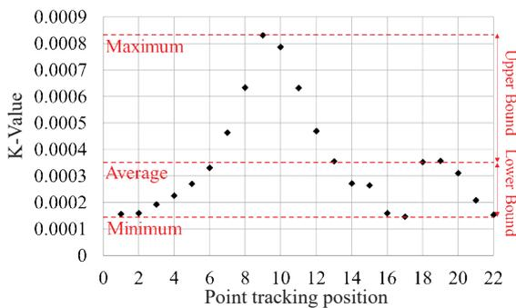
**Figure 22:** Wear coefficient (K) distributions at the different local point.
