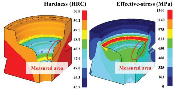
**Figure 15:** Results of the lower die at the finished stage, (a) Hot hardness and (b) Effective stress.
