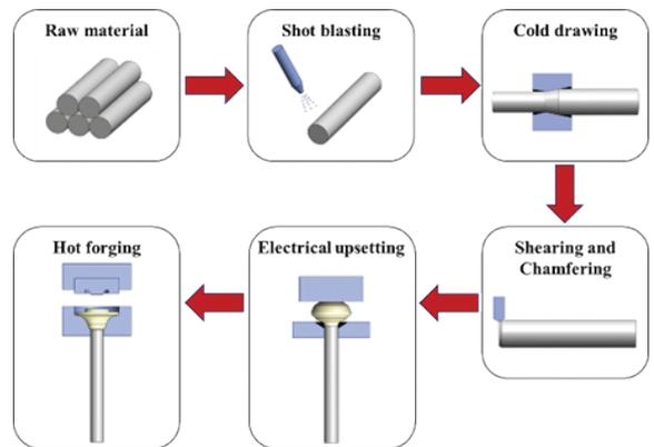
Figure 1: Hot forging process of the axle shaft.
