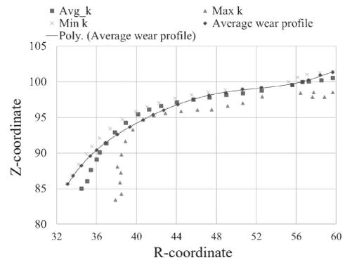
**Figure 23:** Comparison of die wear distributions with different wear coefficient (K-value).
