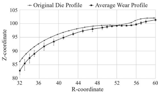
**Figure 10:** Comparison between the original die and average wear profile of the lower die.
