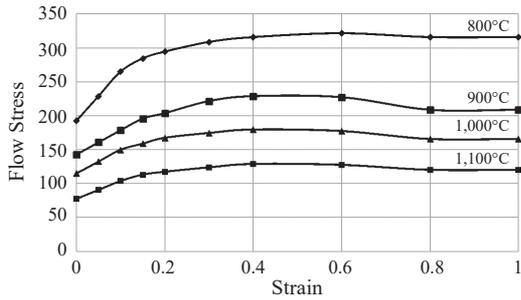
**Figure 13:** Flow stress curve of AISI 1045 at different temperatures.
