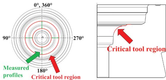
**Figure 9:** Measurement location of die wear profile at the lower die, a) top view and b) side view.
