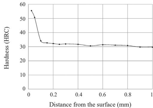
**Figure 6:** Hardness profile of the die after heat treatment and tempering.
