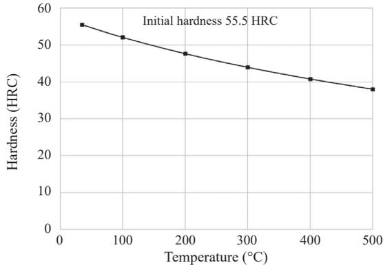
**Figure 14:** Hot hardness profile of die material.
