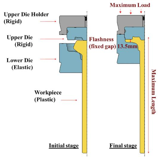
**Figure 12:** Schematic of the simulation model.
