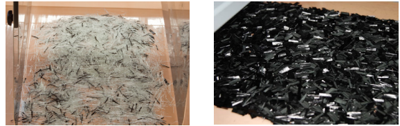
Figure 18: Cutting result of the Cutter; left: mix consisting of Carbon fibers and Glass fibers, right: 50k Carbon fibers.
