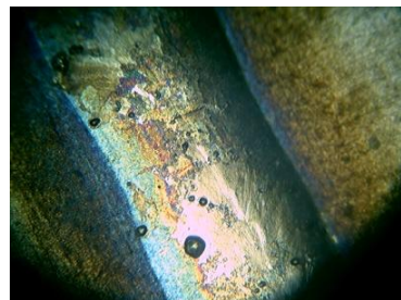
Figure 2d: welding speed of 300 mm/minute
