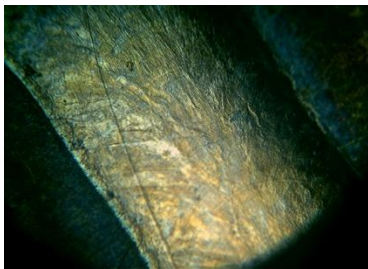
Figure 2a: welding speed of 150 mm/minute
