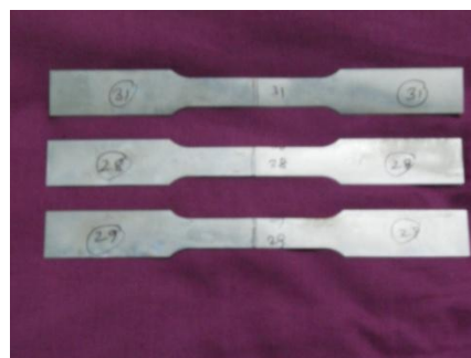
Figure 11: Tensile specimens of AISI 304L welded joints
