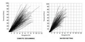
**Figure 4**: Tenacity vs. Elongation of Spanish broom fibres extracted through different methods (extracted from [27]).
