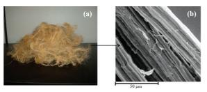
**Figure 3**: (a) Spanish broom fibres extracted by physico-chemical process; (b) SEM micrograph (1000x magnification) [10].
