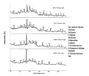
Figure 10: XRD Analysis of LCGPC Mixes.
