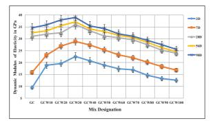
Figure 8: Dynamic elastic modulus of LCGPC.
