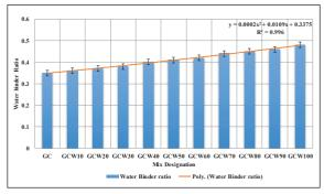
Figure 4: Standard consistency of LCGPC.
