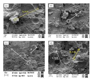
**Figure 9**: Microstructure analysis of LCGPC mixes (a) GCW0 (b) GCW100 (c) GCW10 (d) GCW30.
