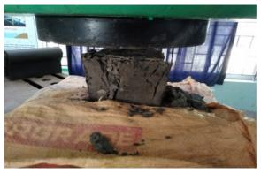
Figure 1: Compressive strength of the LCGPC cubical specimens.
