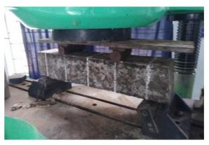
Figure 2: Flexural strength of LCGPC prism specimens.
