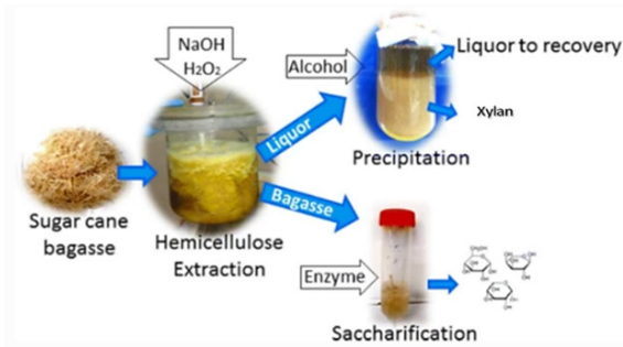
Figure 9: Chemical retting process of sugar cane [29].
