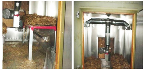
Figure 10: Enzymatic retting process. Flax stalk on shelf in retting/drying chamber (left) and ductwork within chamber (right) [37].
