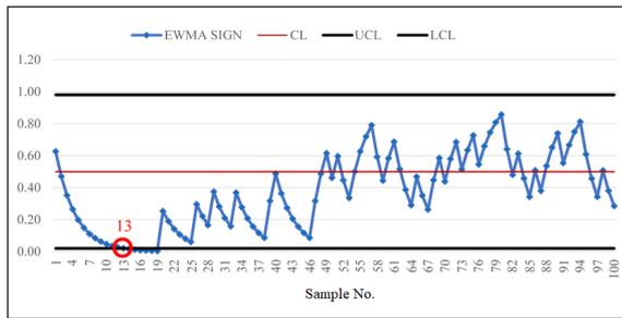
**Figure 5:** Graphical displays of the illustrative of the mine explosion period in the UK during 1875–1951 of EWMA-Sign control chart.
