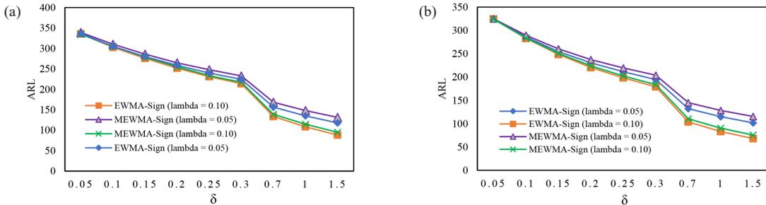
**Figure 1:** ARL of EWMA-Sign and MEWMA-Sign charts for Laplace(1,1) distribution by varying  $n$ : (a)  $n = 5$  and (b)  $n = 10$ .
