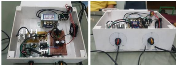
**Figure 6:** Signal amplifying unit and input/output frequency.
