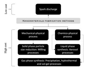
Figure 6: Nanomaterials manufacture methods.
