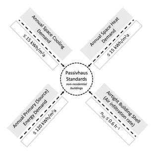
Figure 1: Passivhaus requirements/standard for non-residential buildings.
