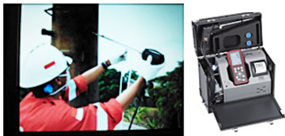
Figure 7: Gas analyzer used to measure emitted gases from the stack.
