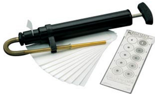
Figure 6: Smoke opacity measurement equipment based on ASTM D 2156-2003.
