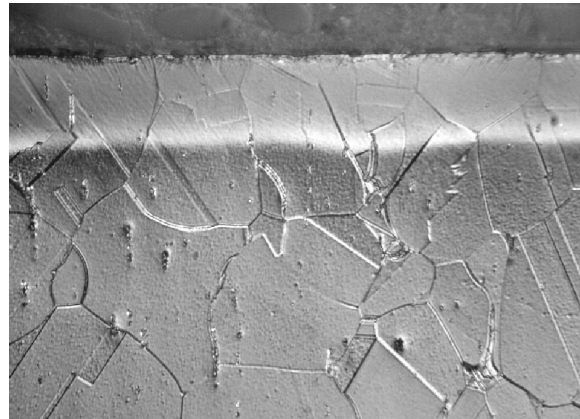
Figure 5: Microstructure in the hardened zone of stainless steel AISI 316L after Kolsterising. Light microscopy in angular light
