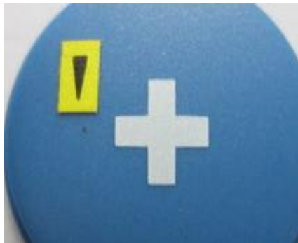
(B) Rejected parts, Black dot dimension bigger than 0.2 mm.
