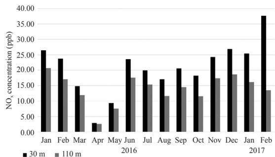
**Figure 3:** NO<sub>x</sub> concentration in urban area at 30 m and 110 m above ground.
