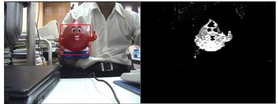
Figure 5: The normal and target-probability views as CAMshift tracks the coloured doll.
