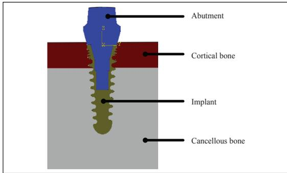
**Figure 1:** Three-dimensional geometrical model of dental implant prosthetic and the surrounding bone.
