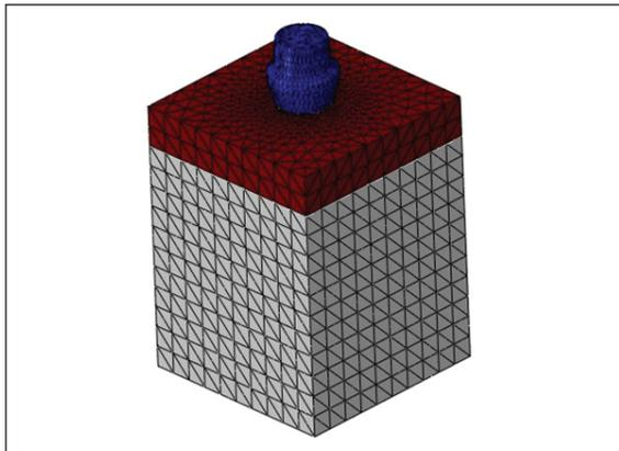
**Figure 4:** The three-dimensional finite element analysis model of the dental implant systems.
