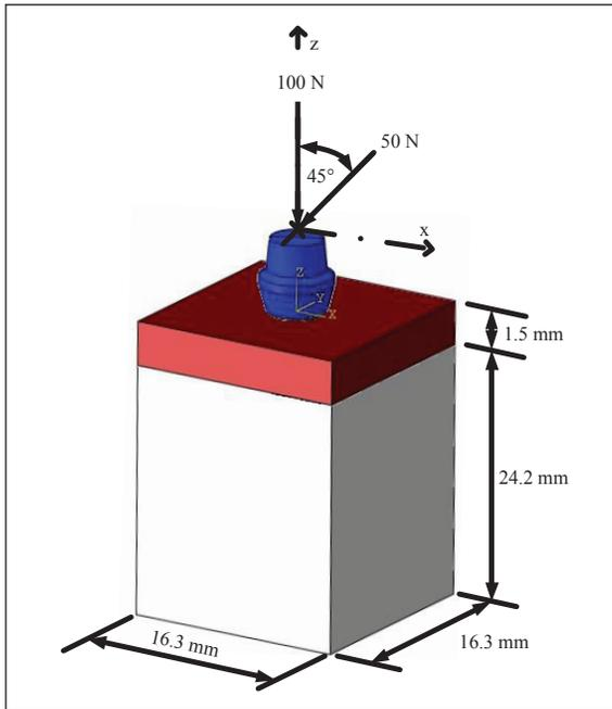
**Figure 3:** Loading conditions applied on dental implant system model.
