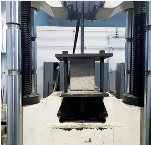
Figure 3: Pull-out test on specimen.
