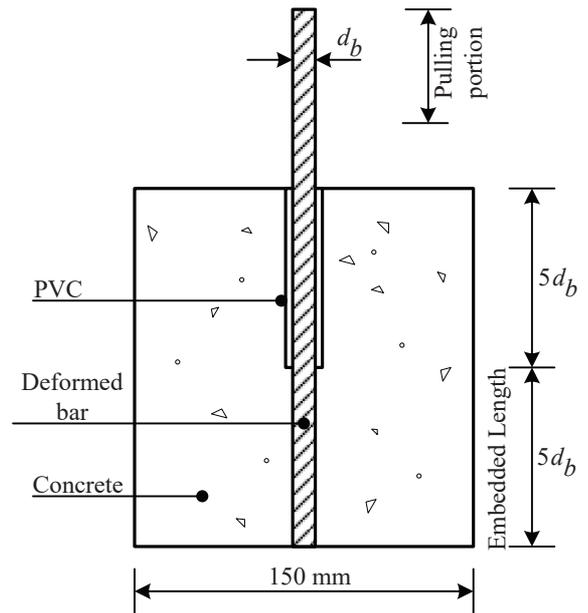
Figure 1: Pull-out test setup.
