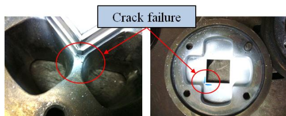
Figure 3: Crack failure in the porthole die [2]
