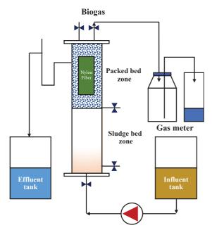
**Figure 2**: The scheme of hybrid reactor used in this study (modified from Suraraksa and Nopharatana [22]).
