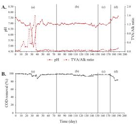
**Figure 6**: A. Changes of pH levels and TVA/Alk ratio, and B. COD removal (%) in hybrid reactor at (a) HRT 7 day with OLR 2 gCOD/L/day (b) HRT 5 day with OLR 2.8 gCOD/L/day (c) HRT 5 day with OLR 5 gCOD/L/day (d) HRT 5 day with OLR 5 gCOD/L/ day (recirculation).
