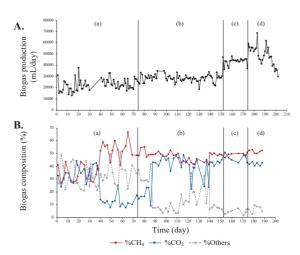
**Figure 5**: A. Biogas production (mL/day) and B. Biogas composition (%) in hybrid reactor under different conditions. (a) HRT 7 day with OLR 2 gCOD/L/day (b) HRT 5 day with OLR 2.8 gCOD/L/day (c) HRT 5 day with OLR 5 gCOD/L/day (d) HRT 5 day with OLR 5 gCOD/L/day (recirculation).
