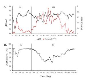
**Figure 4**: A. Changes of pH levels and TVA/Alk ratio, and B. COD removal (%) in hybrid reactor (a) at HRT 20 day with OLR 0.5 gCOD/L/day and (b) at HRT 10 day with OLR 1.4 gCOD/L/day.
