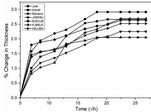
**Figure 12:** Thickness swelling characteristics of the investigated composites with individual fibres and various stacking sequences in the hybrid configuration.
