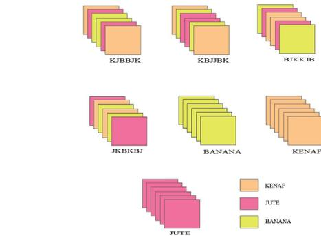
**Figure 1:** Layering arrangements of Banana, Jute and Kenaf fibre mats.
