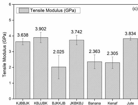
**Figure 7:** Tensile Modulus of investigated composites with individual fibres and various stacking sequences in the hybrid configuration.
