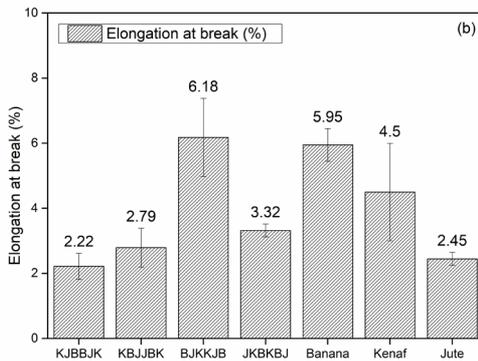
**Figure 6:** Elongation at break of investigated composites with individual fibres and various stacking sequences in the hybrid configuration.
