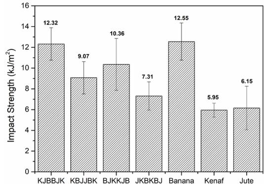
**Figure 10:** Impact strength of investigated composites with individual fibres and various stacking sequences in the hybrid configuration.
