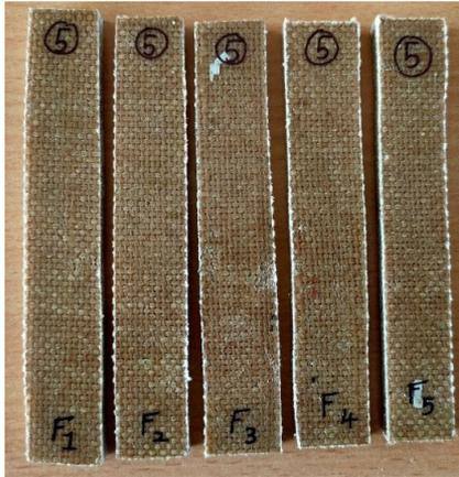
Figure 3: Sample specimen used in flexural test.
