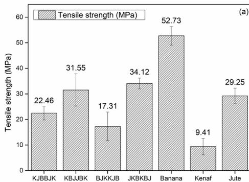
**Figure 5:** Tensile strength of investigated composites with individual fibres and various stacking sequences in the hybrid configuration.
