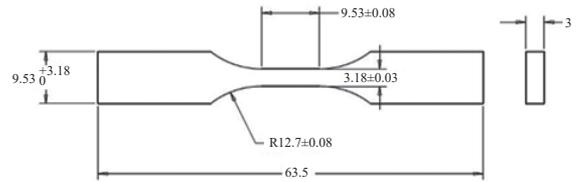
**Figure 2:** D638 ASTM standard type V tensile test sample.
