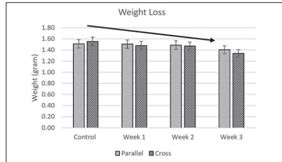
**Figure 7:** Mass loss graph in post-weathering and control specimens.
