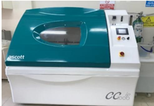
**Figure 4:** Weathering test cabin.
