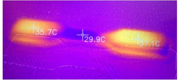
**Figure 9:** Thermal image of the cooling in the sample after FFF printing.
