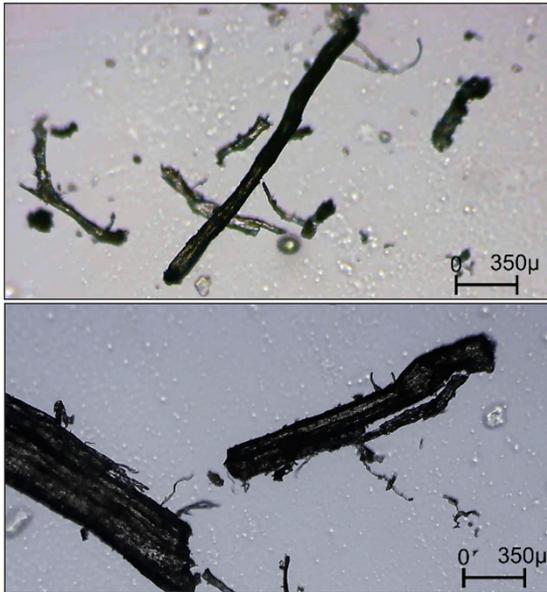
**Figure 1:** Optical microscope photo of hemp fibers.
