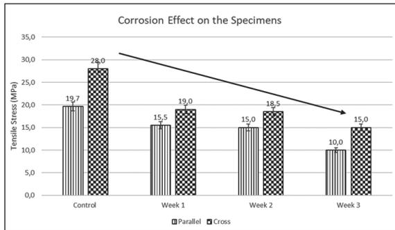
**Figure 6:** Tensile strength values after weathering and control specimens.
