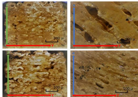
**Figure 8:** Optical microscope images of 3D printing specimens (Upper +/- 45, bottom parallel).
