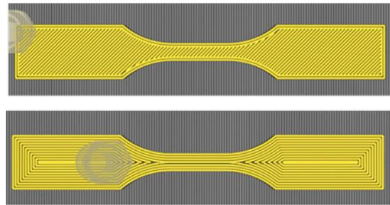
**Figure 3:** Infill patterns geometries, (upper  $\pm 45^\circ$ , bottom linear).
