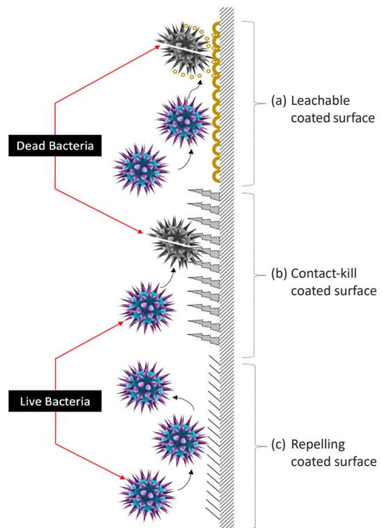
**Figure 5:** Antibacterial surfaces are classified as (a) Leaching antibacterial agents, (b) Contact-kill bacteria, and (c) Prevent bacteria adhesion.
