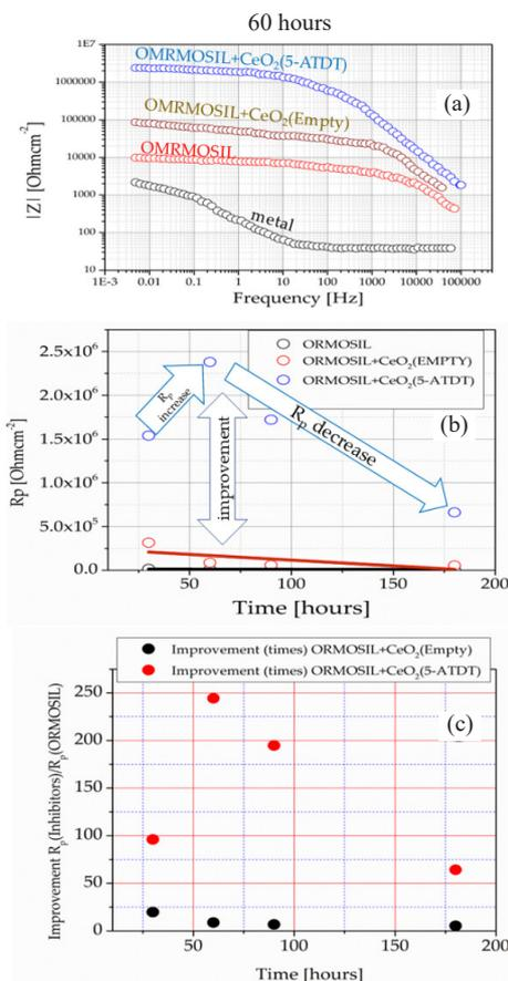
**Figure 2:** (a) EIS of all samples exposed to salt water for 60 h. (b)  $R_p$  of the HDG + ORMOSIL, HDG + ORMOSIL +  $\text{CeO}_2$ (EMPTY) and HDG + ORMOSIL +  $\text{CeO}_2$ (5-ATDT) coatings as a function of the exposure time in salt water. (b) Improvement of  $R_p$  of HDG + ORMOSIL +  $\text{CeO}_2$ (EMPTY) and HDG + ORMOSIL +  $\text{CeO}_2$ (5-ATDT) compared to  $R_p$  of HDG + ORMOSIL (c).
