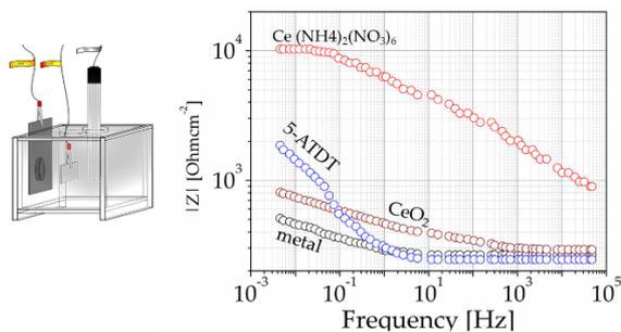
**Figure 1:** Nyquist diagram after 30 hours of exposure of HDG steel in a 0.05 M NaCl corrosive environment and the same corrosive environment with corrosion inhibitors.
