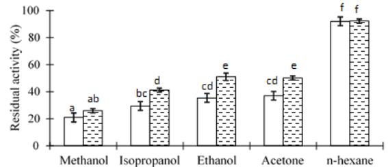
**Figure 6:** Effects of organic solvents on the activity of free (□) and immobilized (▨) lipases. Note: Different letters indicate significant differences among samples ( $p < 0.05$ ).
