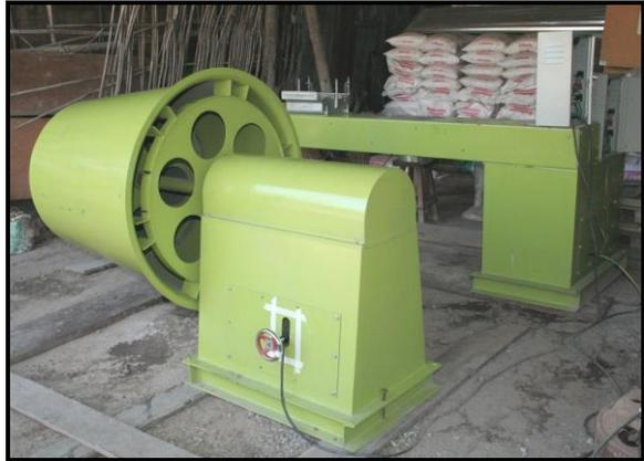
**Figure 3:** Automatic fiberglass winding machine [3]
