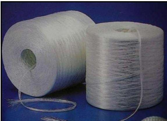
**Figure 2:** Fiberglass yarn
