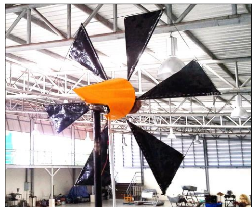
Fig.2 Downwind Thai sail windmill [3]
