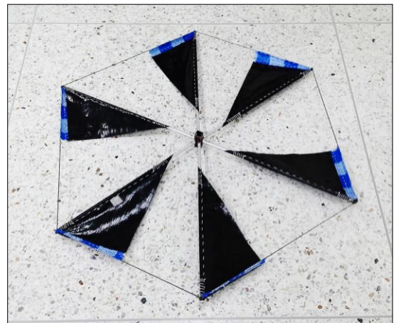
Fig.8 The 6-blade rotor by using the technique of closing the blade tip (Closed-tip DTSW)
