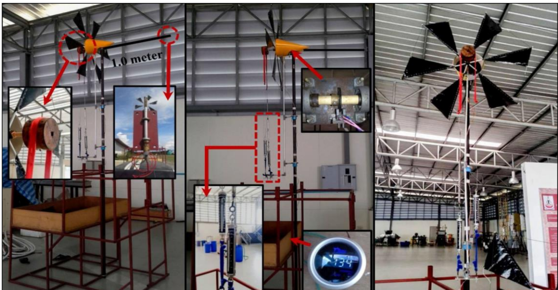
Fig.9 Carbon steel rack, prototypes, and measurement accessories installation: tension spring, optical rotational speed sensor, and anemometer [3]
