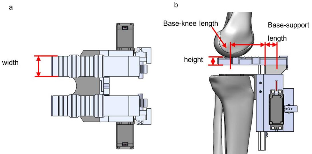
**Fig. 1** The knee position with the main parameter consists of 4 factors such as width, height, base-knee length, and base-support length: (a) top view and (b) side view
