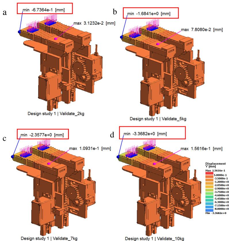
**Fig. 8** The FEM simulation result of the new beam bending displacement in each load of the beam:
