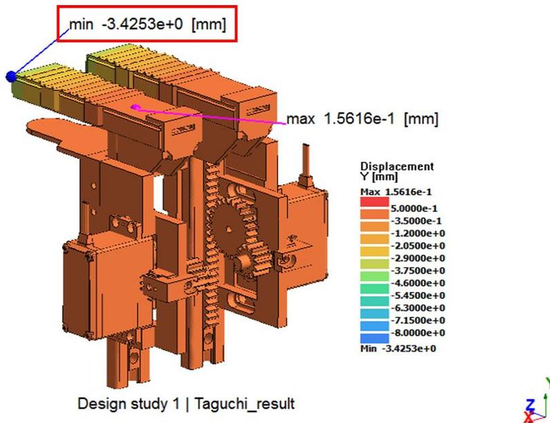
Fig. 6 The FEM result of bending displacement of the parameter from Table 8
