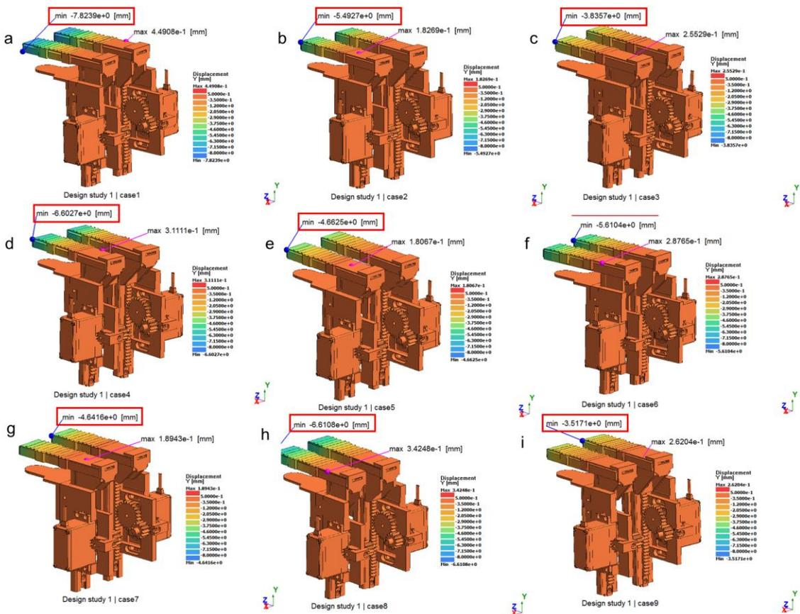
**Fig. 4** The FEM simulation in the y direction of the model beam from Table 4: (a) experiment 1, (b) experiment 2, (c) experiment 3, (d) experiment 4, (e) experiment 5, (f) experiment 6, (g) experiment 7, (h) experiment 8 and (i) experiment 9
