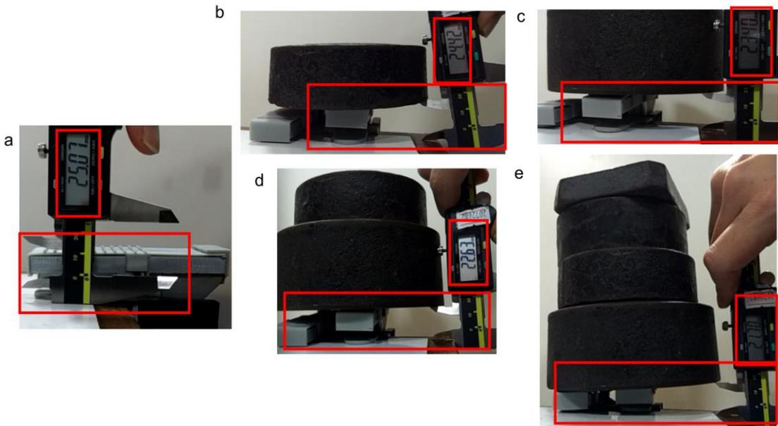
**Fig. 7** (a) The initial displacement without load measuring 3 times in a row with a digital vernier caliper and the (b) measuring bending displacement with loads of 2 kg, (c) 5 kg, (d) 7 kg, and (e) 10 kg
