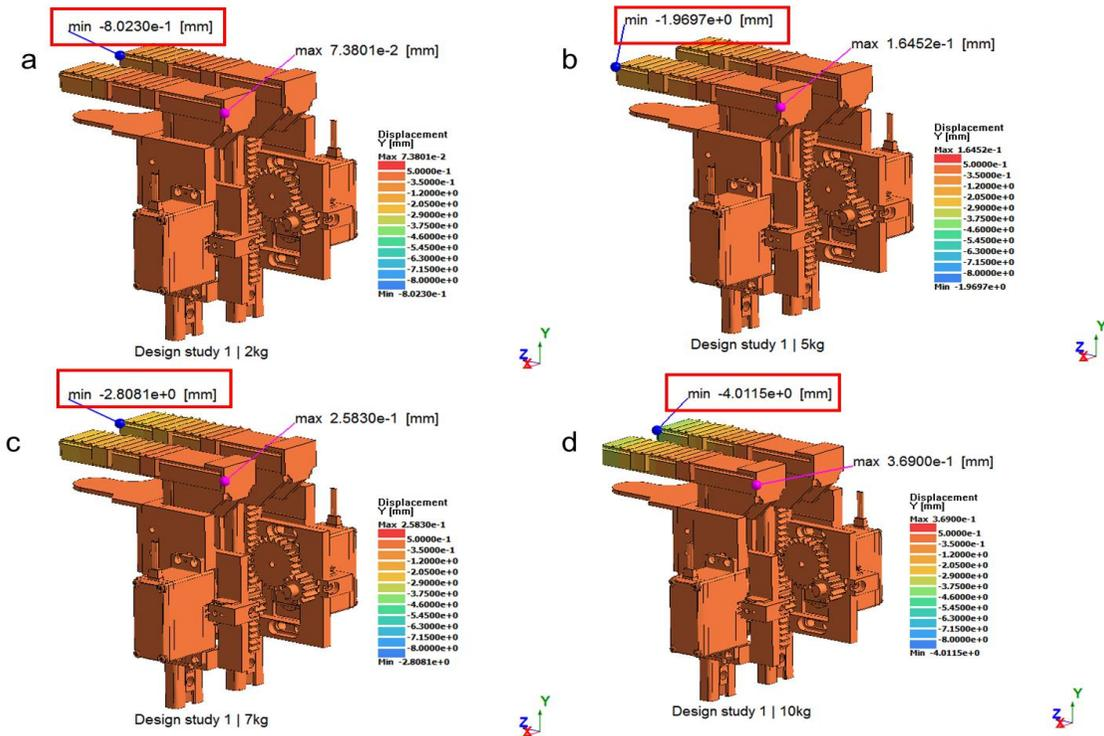
Fig. 3 The FEM simulation result of bending displacement in each load of the beam:
