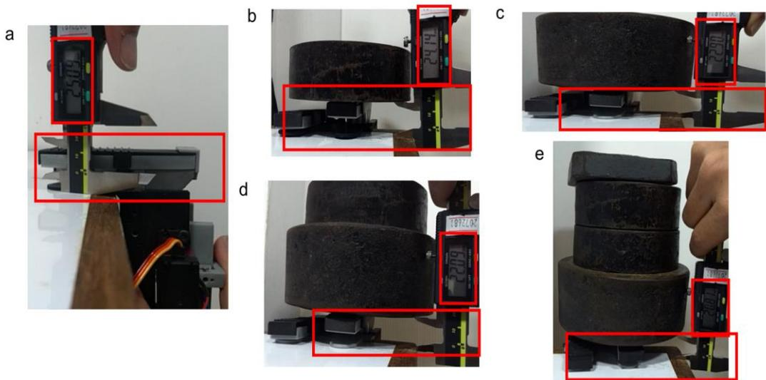
**Fig. 2** (a) Initial displacement without load measuring 3 times in a row with a digital vernier caliper and (b) the measuring displacement of the beam with loads at 2 kg and (c) 5 kg
