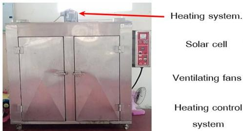
**Fig. 2** The former three-phase electric oven
