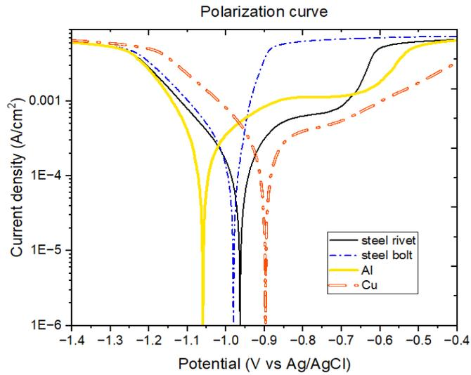
**Fig. 8** Polarization curves of Al A1050, Cu C1100, bolt, and steel rivet
