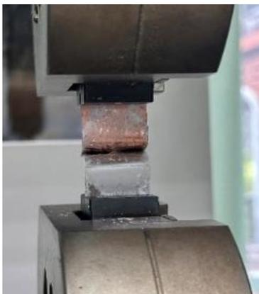
**Fig. 3** T-peel shape test in UTM alignment
