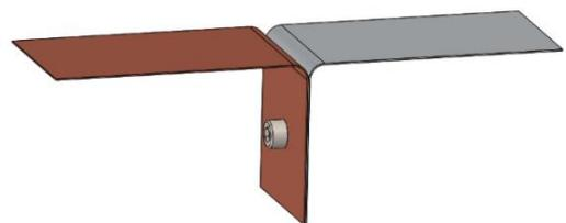
**Fig. 1** Geometrical illustration of T-peel shape workpiece
