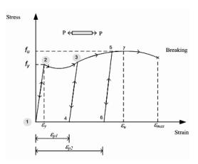
Figure 1 Typical stress-strain curves of mild steel
