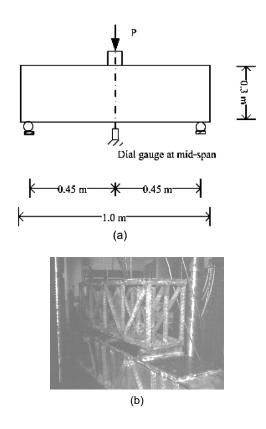
Figure 10 Typical test set-up for 1.0 m truss
