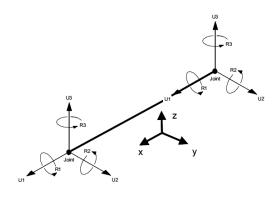
Figure 4 Frame element with six DOF at each end
