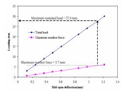
Figure 7 The relation between the maximum member forces, total load and the midspan deflection of 1.0 m truss
