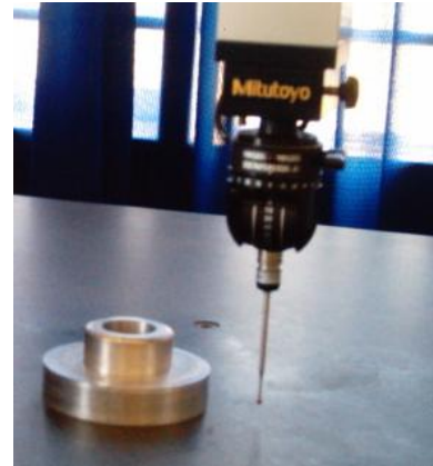
Figure 3: Measuring cam profile on the Mitutoyo Beyond Crysta 554 CMM machine
