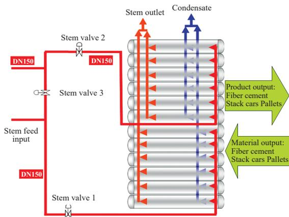
**Figure 4:** The autoclave system layout.
