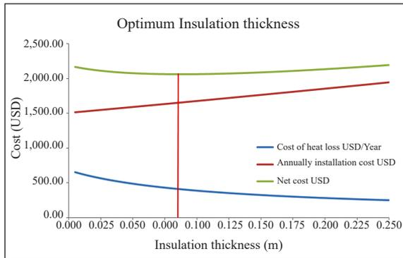
**Figure 6:** Finding the optimum insulation thickness of the autoclave in USD.
