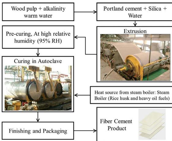
**Figure 1:** Fiber cement Process diagram [1].
