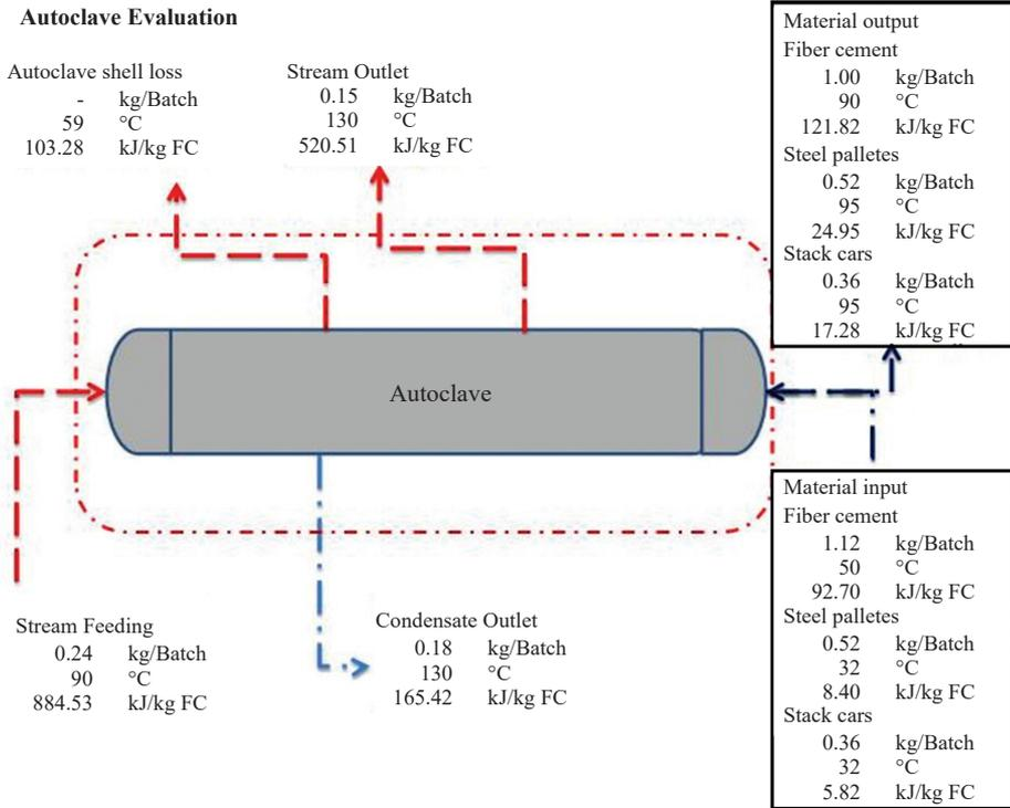
Figure 5: Analysis of heat and mass of normal operation autoclave.
