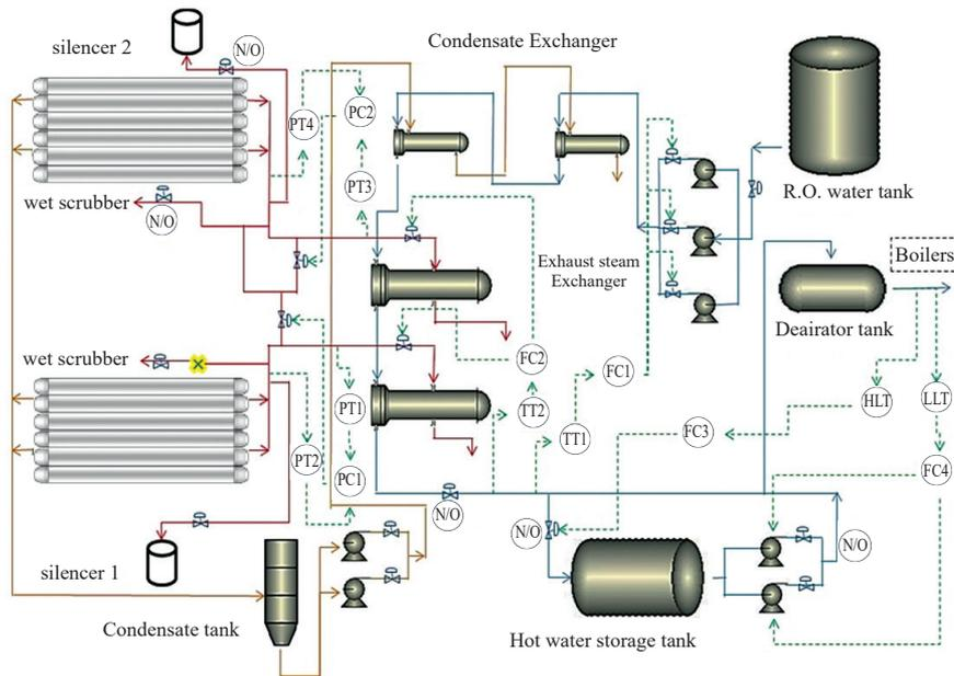
**Figure 8:** Process flow and instrument diagram of the Waste heat recovery system.
