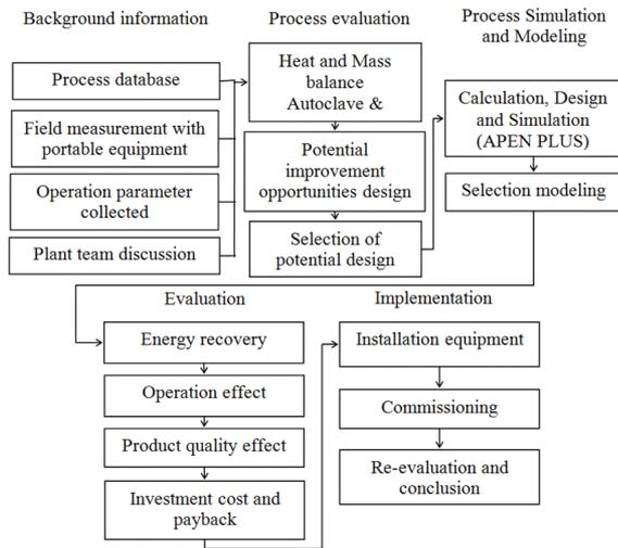
**Figure 2:** Implementation of heat recovery diagram.
