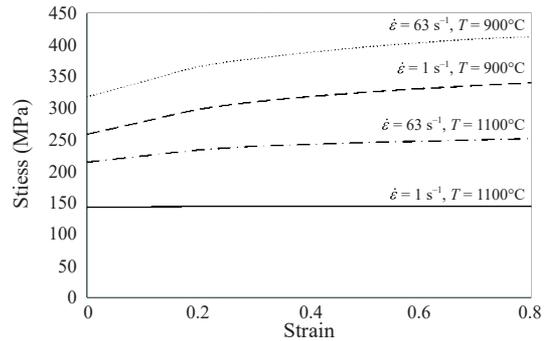
**Figure 4:** Material property of AISI 316L stainless steel at different temperatures and strain rates.
