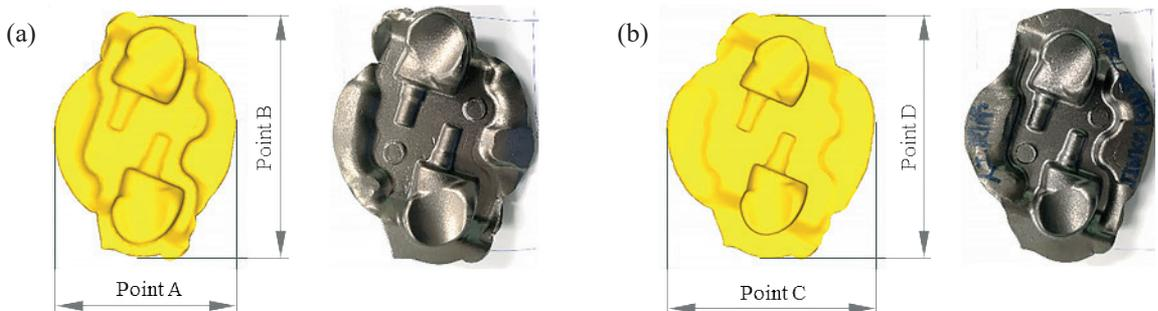
**Figure 8:** Comparison of the geometrical shapes after forming between the FEM and the experiment at (a) roughing step, and (b) finishing step.
