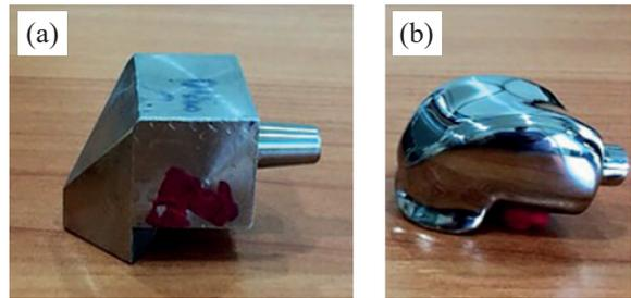
**Figure 1:** (a) Preform shape of the talar body prosthesis for the manual grinding process, and (b) the talar body prosthesis after the cutting and the manual grinding process.
