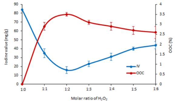
**Figure 2:** Effect of H<sub>2</sub>O<sub>2</sub> molar ratio on OOC and IV values.
