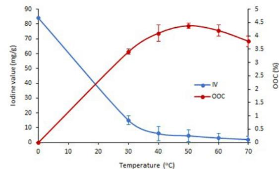
**Figure 4:** Effects of reaction temperature on OOC and IV values.
