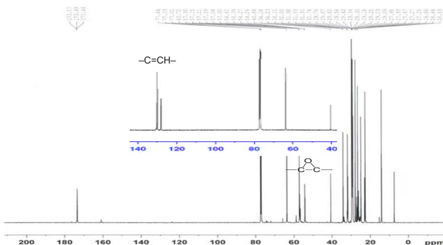
**Figure 8:**  $^{13}\text{C}$  NMR spectra of TMPJO (inserted) ETMPJO triester.
