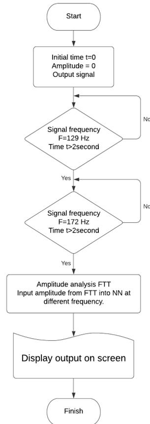
Figure 4: Programming process for watermelon sorting operation.
