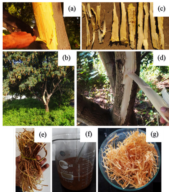
Figure 1: (a) and (b) Pithecellobium dulce (PD) bark tree, (a) and (d) Peeling of PD tree skins, (c) PD skins (e) Peeled PD fibers, and (f) and (g) Skin tipped in NaOH solution and dry PD fibers.
