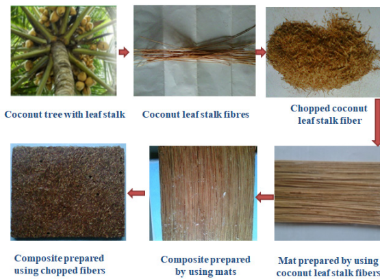
Figure 2: Fabrication procedure of the composites.
