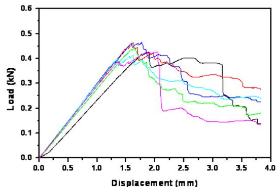
**Figure-8:** Load-displacement curves of 2wt% CNF and 2.5wt% ETBN composites
