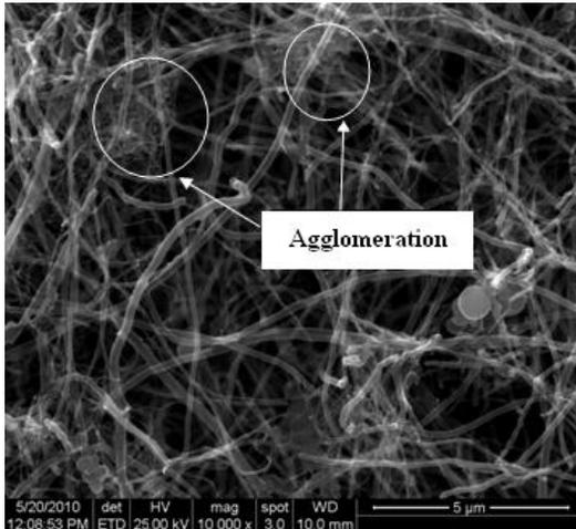
**Figure-1:** SEM image of carbon nanofibers showing agglomerates.
