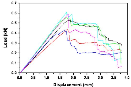
**Figure-7:** Load-displacement curves of 1wt% CNF and 2.5wt% ETBN composites
