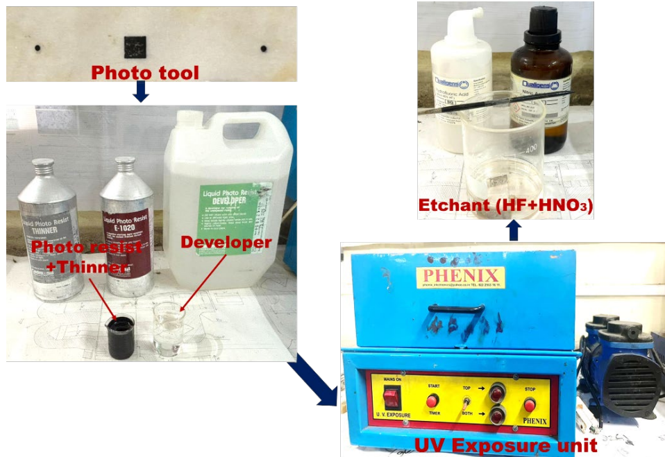
Figure 1: Experimental setup employed for PCM machining of Ti-6Al-4V alloy.
