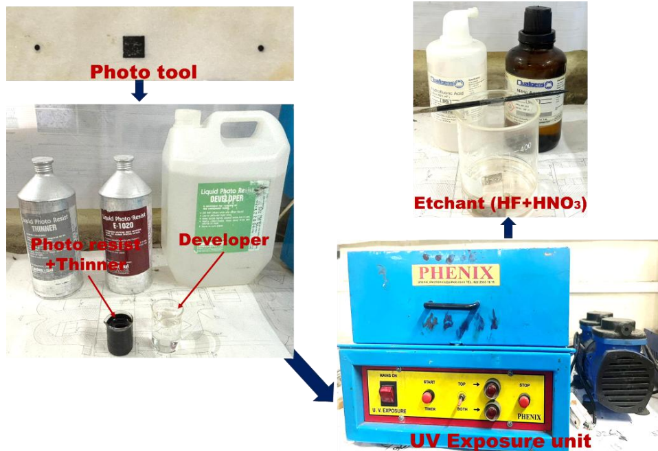
Figure 1: Experimental setup employed for PCM machining of Ti-6Al-4V alloy.
