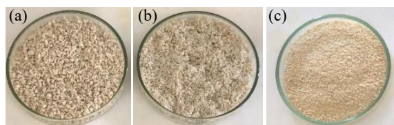
Figure 2. Preparation of samples. (a) OPEFB cellulose before homogenization; (b) OPEFB cellulose after homogenization; (c) CMC OPEFB.
