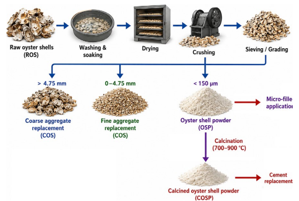
Figure 4: Preparation and processing pathways of oyster shells for concrete applications.
